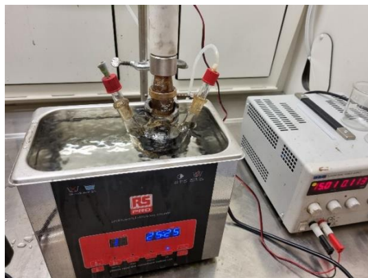
Figure A.1, The three-way flask is kept within the heater and sonification bath.
