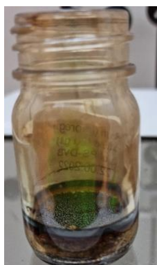
Figure 4.2, Impregnated resins via normal method after 15 days being left with an open flask.
