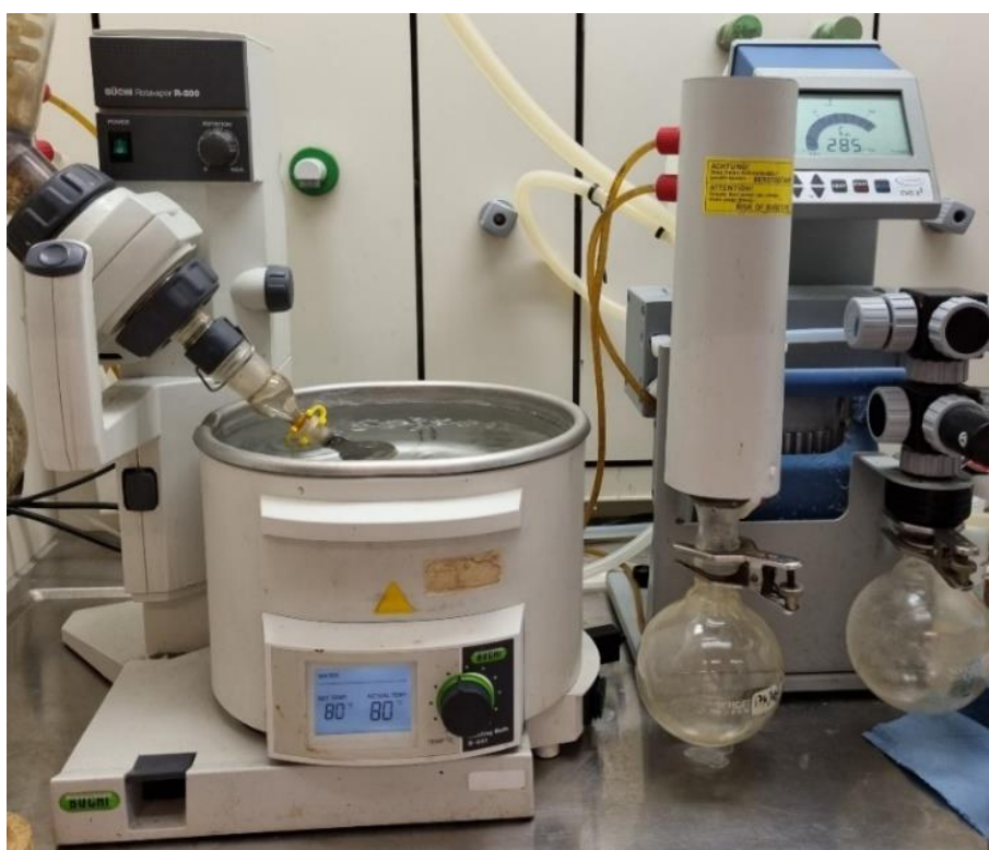
Figure 3.2, the rotary evaporator laboratory setting with a heating bath containing a flask.
