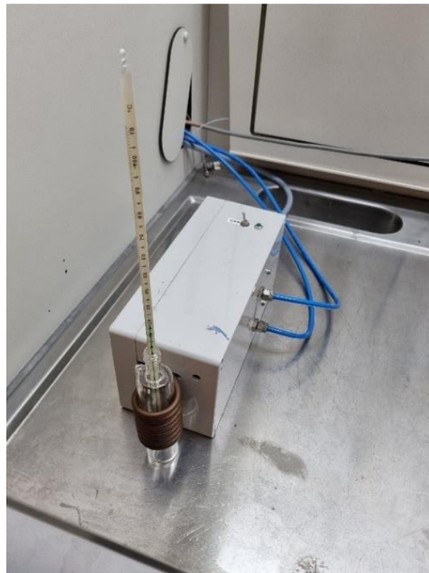
Figure 3.7, the external AMF for the hyperthermia studies is produced by solenoid.
