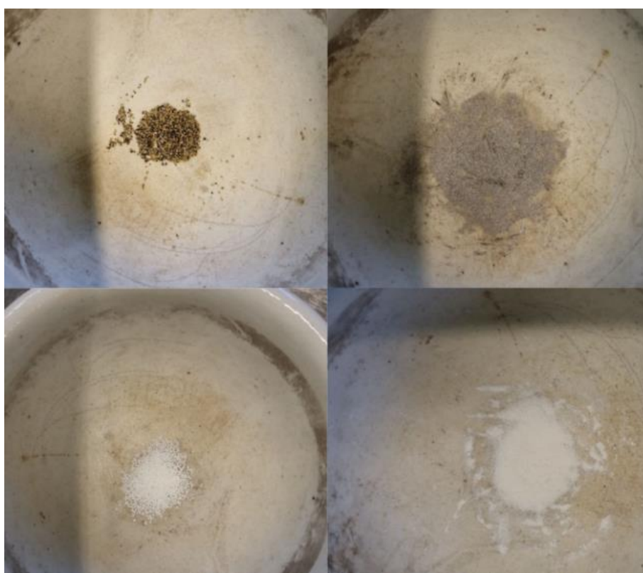
Figure 4.1, Visual confirmation of impregnation via intensified method by grinding the particles.
