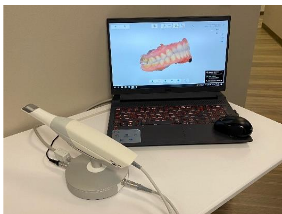
Figure 2.4. The 3Shape (Copenhagen, Denmark) Trios 3 intraoral scanner. 14
