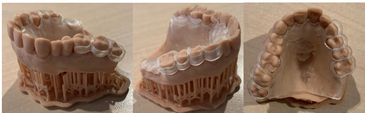
Figure 4.14. 3D-printed baseplate and retention clasps fitted on a 3D-printed dental cast. The clasps are evaluated according to the design criteria stated in Table 4.4.
