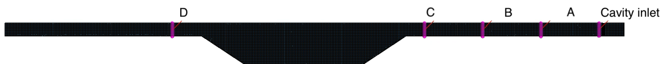
Figure 3.13. Line probes placement along the cavity. Locations of the line probes relative to the cavity downstream end (Cavity inlet: 3.04 m, A: 2.74 m, B: 2.44 m, C: 2.14 m and D: 0.84 m)
