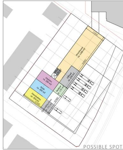
Figure 2.2 – Dimensions of new warehouse
