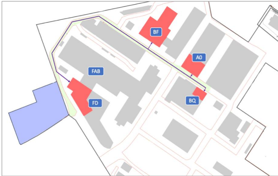
Figure 1.2 – Map of ICN8 plant where the warehouses are in red and the paths between the warehouses in blue.
