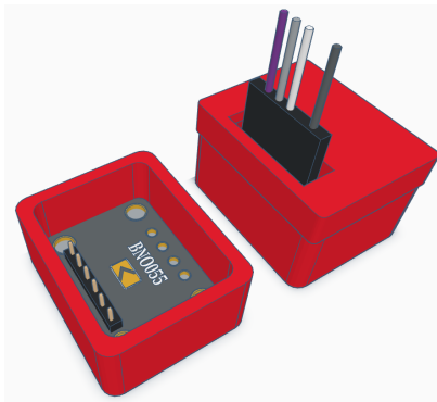
Fig. A5: IMU (Adafruit BNO055) in 3D-printed casing. Used in the Posture protocol.
