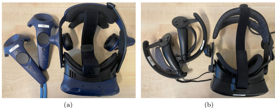
Figure 11: The Figure on the left shows the HTC Vive headset with controllers 21 , and the Figure on the right demonstrates the Valve Index with controllers 22
