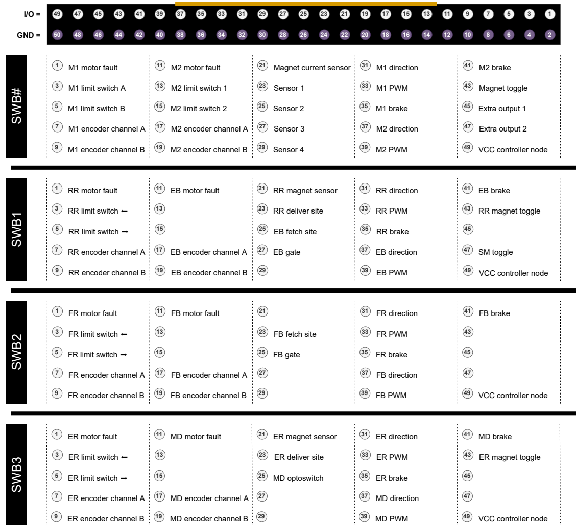
Figure A.7: Definitions of the 50-pin connector on the switch board. For the abbreviation definitions see Figure A.2.
