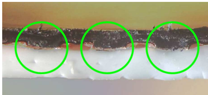
Figure 2.3: A cross sectional view of a sample with EPLA extruded over perforated copper tape on a base layer of PLA. The green circles indicate where polymer has successfully penetrated through the holes and bonded with the base layer [12].
