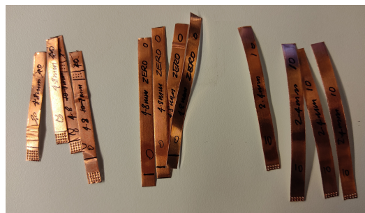
Figure 4.7: A set of tapes with a different number of perforations and identification markers. Shown here from the left are tapes of 20, 0 and 10 holes, with 4.8 mm being the length of the tape to be enclosed by the polymer.
