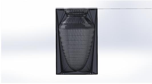
Figure 3: Design of the outer mold for the left ventricle, representing normal dimensions for healthy men. This mold is needed in duplicate to create the entire outer cast for the left ventricle.
