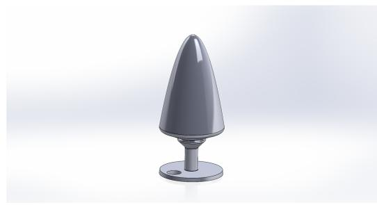
Figure 4: Design of the inner mold for the left ventricle, representing normal dimensions for healthy men.
