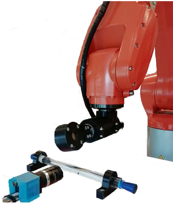
Figure 3: Wireless manipulation system of the KUKA robotic arm with a rotating magnetic field attached.
