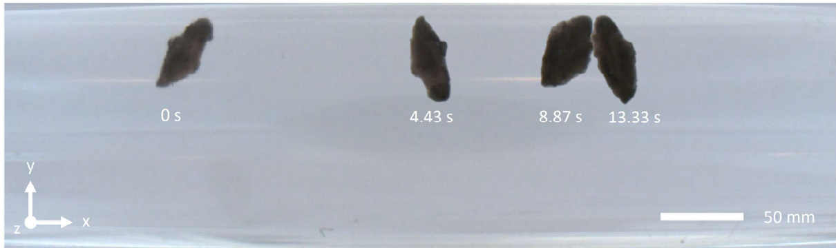
Figure 4: Actuation of an IRONSperm cluster with 2 mg/mL nanoparticle concentration at 1.5 RPM frequency. Overtime, the cluster moves along the x direction as the RPM rotates clockwise.
