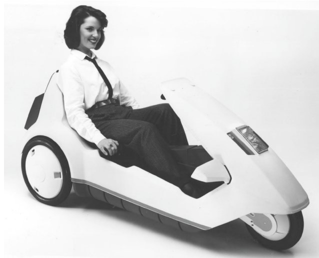
Figure 3.13. Sinclair C5 An electrically assisted pedal tricycle, designed by Sir Clive Sinclair in the 1980s to revolutionize the personal vehicle market with a low-cost and eco-friendly design solution. Despite the sleek and well-intentioned design, the product failed because it lacked practicality and failed to meet user needs. Image from Getty Images
