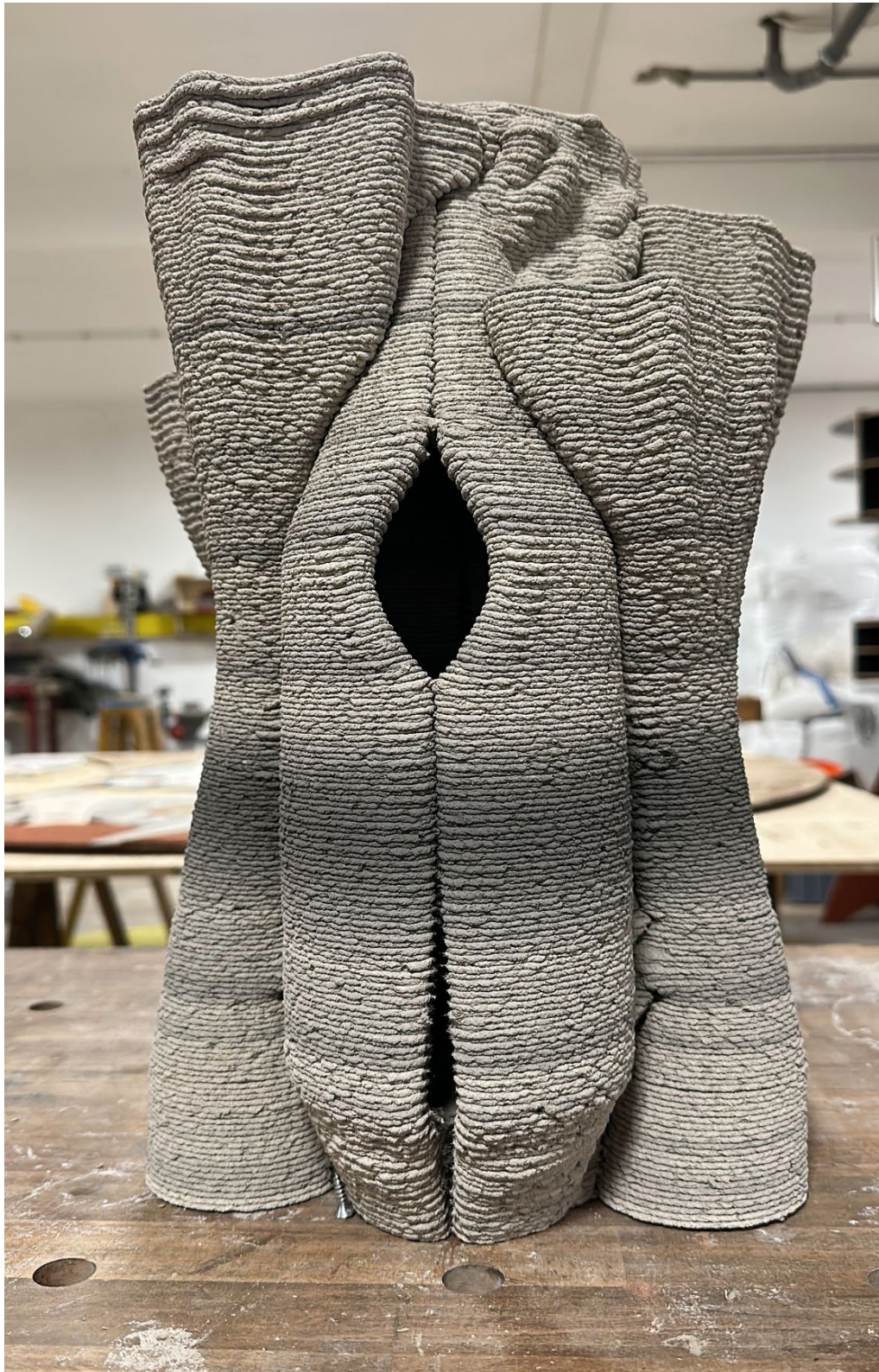
Figure 6.10. Birdbead prototype. Printed and dried Birdbead model with a split in the front, Photo by Huub Looze.
