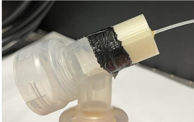
Figure 2.2: Picture of the 3D-printed coupling piece connected to the connector using tape and the tube
