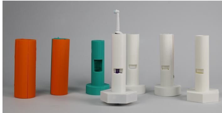
Figure 9.4: Different iterations of 3D printed cases, with the final design in the middle.
