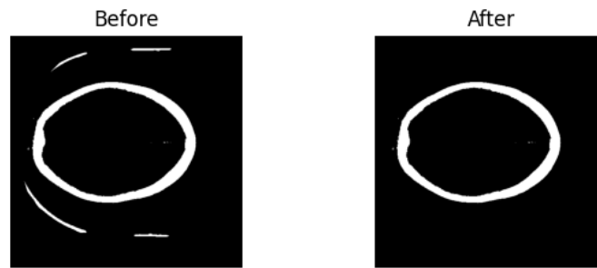
FIGURE 8.3: Before and after keeping the largest component. The left side shows the head fix of the CT machine, which is removed on the right side.
