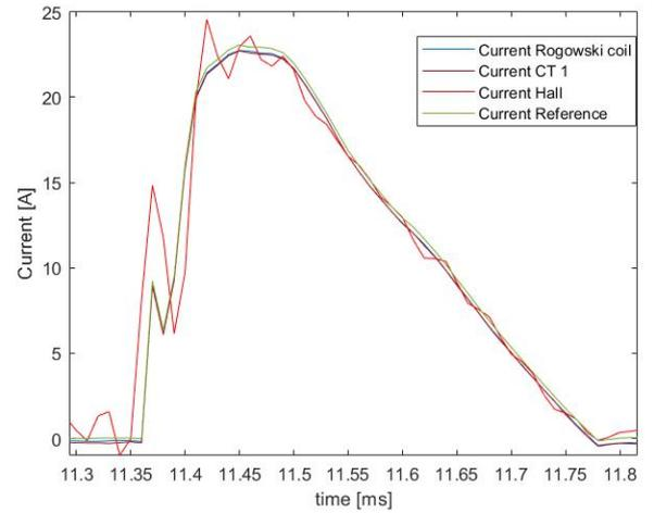
Fig. 11: Zoomed in measured water pump 1 signal
