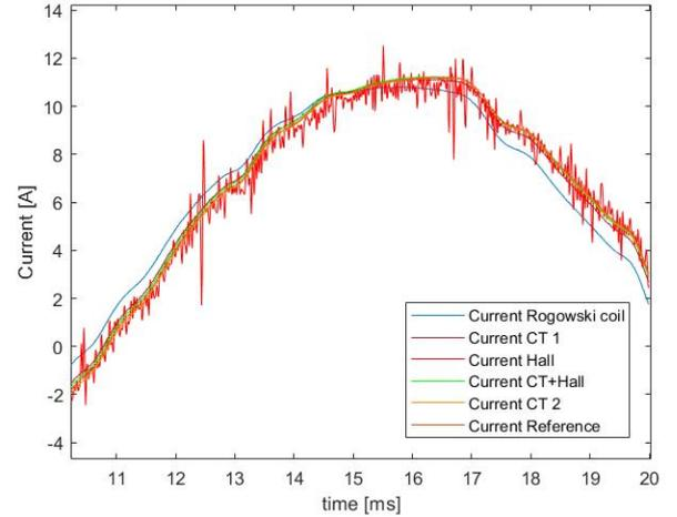
Fig. 9: Zoomed in measured 1800W Heater signal
