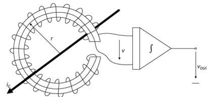
Fig. 3: The operation principle of a Rogowski coil [6].
