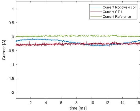
Fig. 12: Zoomed in measured water pump 1 signal of rogowski coil
