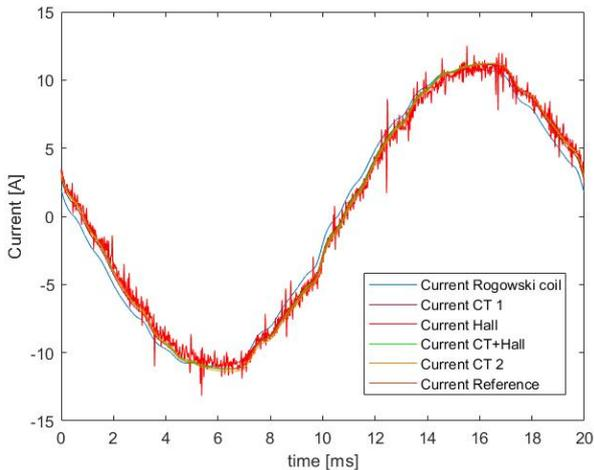
Fig. 8: Measured 1800W Heater signal
