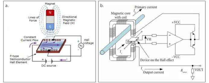
Fig. 1: a. Working principle of a Hall effect sensor. b. A compensation type Hall effect sensor [1].
