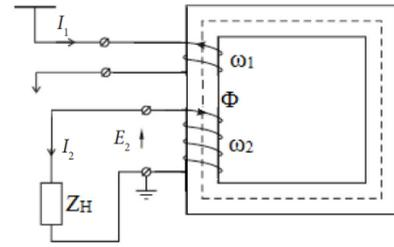
Fig. 2: The operation principle of a current transformer [1].
