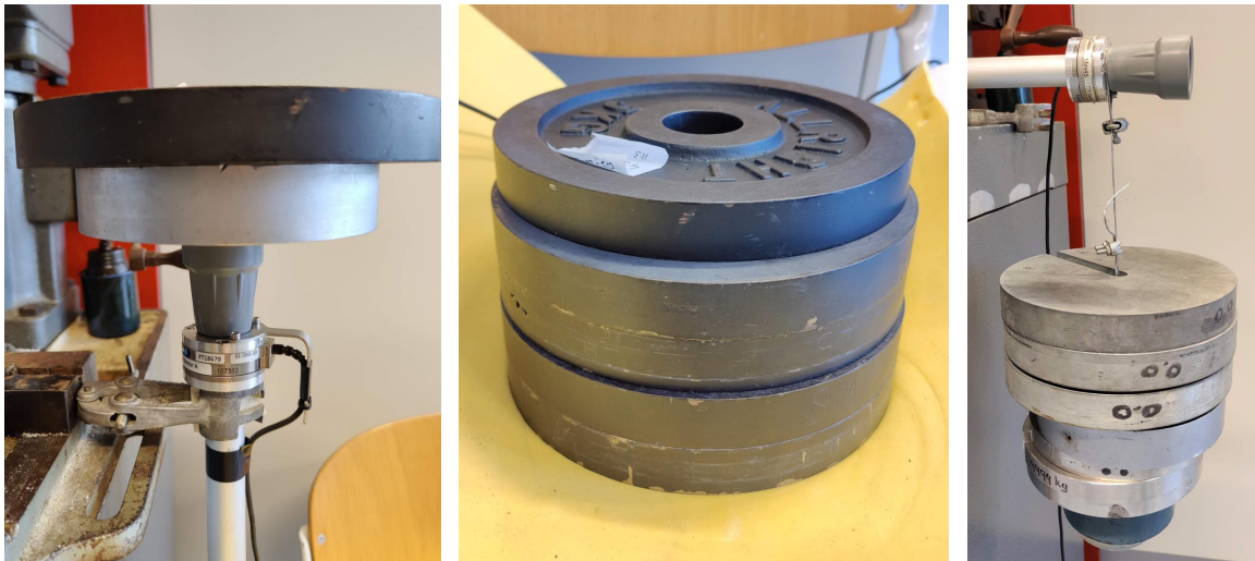
Figure 2.2: Left: Measurement set-up for applying known forces/weights to the sensor in z-direction. Middle: Weights for z-direction measurement. Right: Measurement set-up for applying known forces/weights to the sensor in sideways direction.
