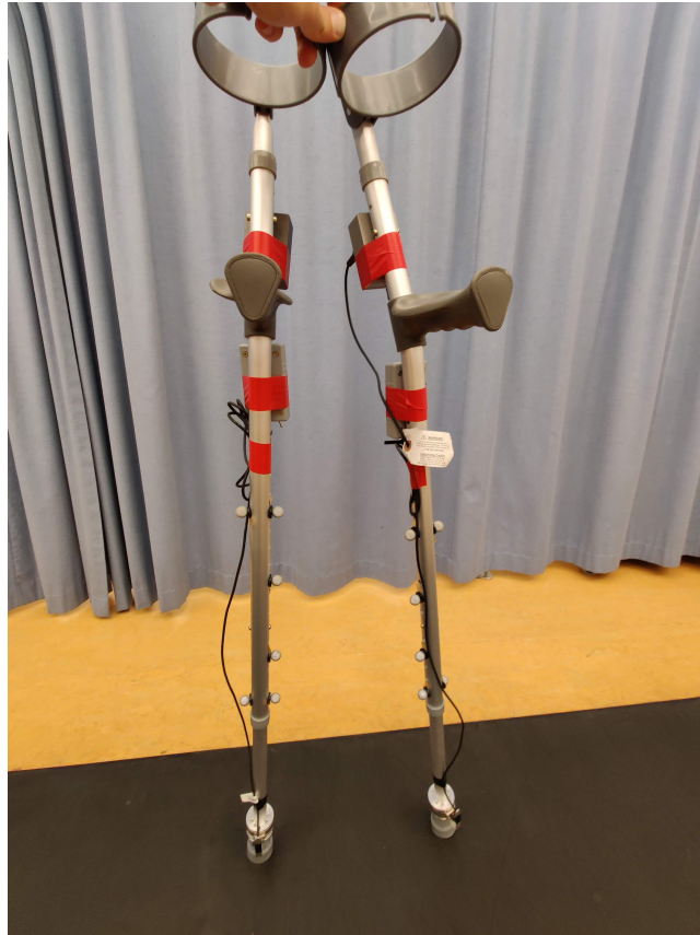
Figure D.2: The crutches in the lab with optical markers for the VICON system attached.
