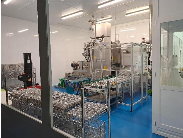
Figure 21: Water-based precision ultrasonic cleaning system
