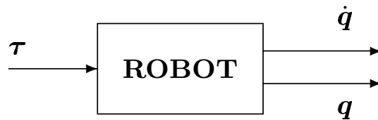
Figure 2.11: Input output representation of a manipulator [9].
