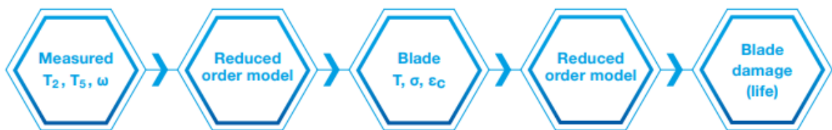
Figure 20: Situation and outline of the underlying models of a turbine blade's digital twin (from [26])
