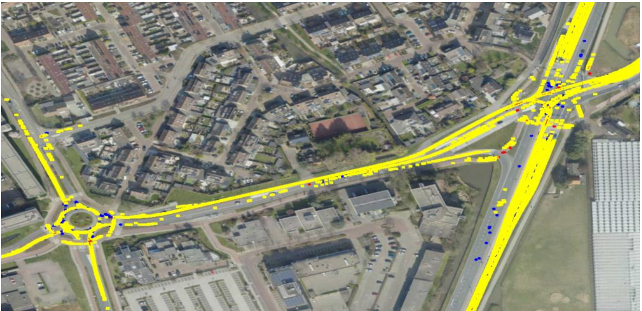
Figure 15 - Overview of the study area with the location of conflicts for the reference scenario sorted by type of conflict (yellow = rear-end, blue = lane change, red = crossing)
