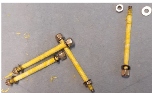
Figure B.3: Metal fasteners wrapped with teflon tape.
