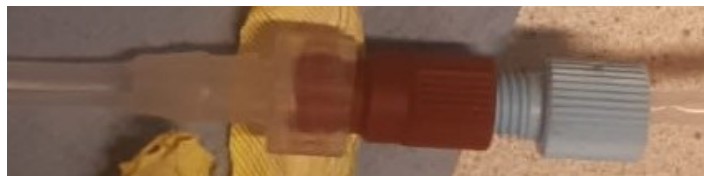
Figure B.2: Barbed adapter (transparent), Luer lock adapter (red), and flangeless fitting (blue).
