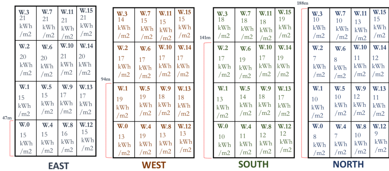
Figure 54 BIPV estimation on Tower A
