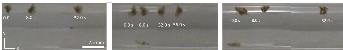
Figure 4: Rolling locomotion of three IRONSperm clusters under the actuation of the RPM with 1.6 Hz. From left to right the concentration of nanoparticles are 1 mg/mL, 2 mg/mL and 3 mg/mL
