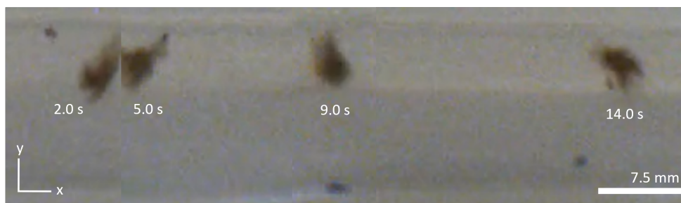
Figure 6: Rolling locomotion of cluster with 1 mg/mL concentration at 1.6 Hz actuation from sample set C. The detached cluster part attaches and increases the velocity.
