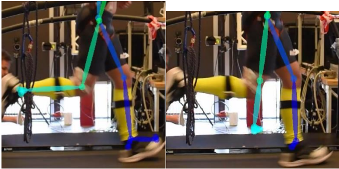
Figure 1.1. two consecutive frames of a jitter error happening.
