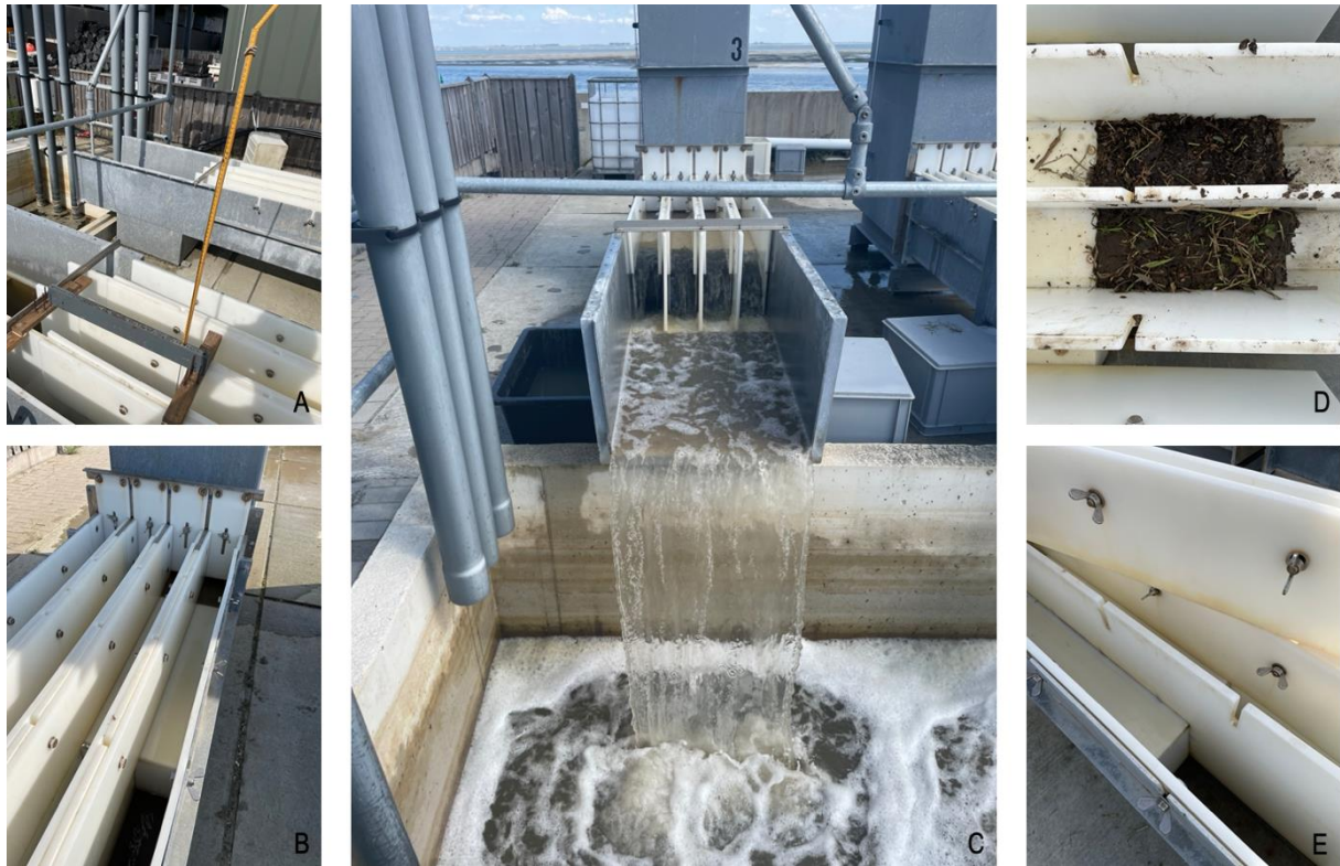
Figure 11 Fast Flow Flume of the NIOZ research institute: A) the height measuring set-up B) the flow regulating plate C) the operating Flume D) two samples placed in the flume E) the boundary reducing alignment plate
