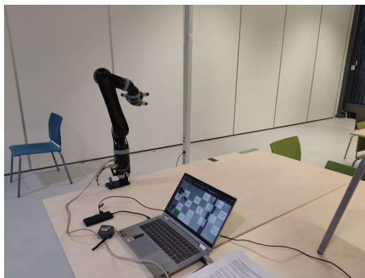
Figure 7.1: The setup used in the experiment to validate the system. The robotic arm is mounted to the table, a safe distance away from the user. A spot around 55 cm was marked for placing objects.
