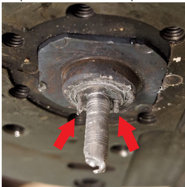
Figure 62: Tool housing at nozzle area with dismantled nozzle plates. Arrows indicating aluminium pushing out thermocouples.
