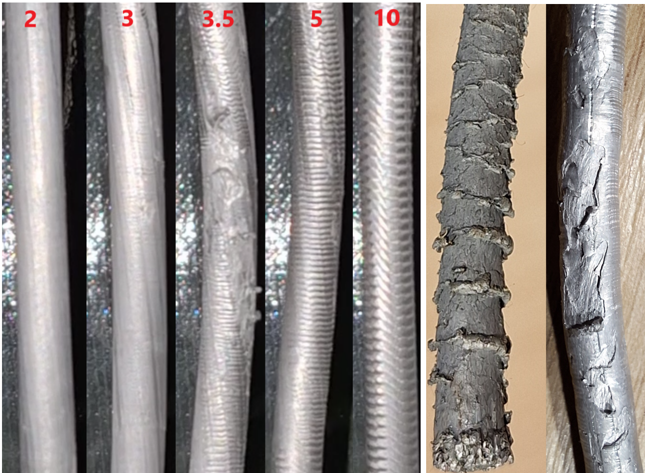
26.a. 2TG3.5_400_x: From left to right increase in feed velocity with gradually changing appearance within the same experiment. Key numbering in red. 26.b. Close-up of palm tree (left) and shark skin (right) extrusion defects
