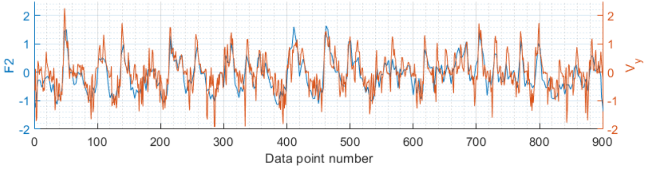
Figure 45: F_2 and V_y data from Figure 44 scaled and plotted over each other.
