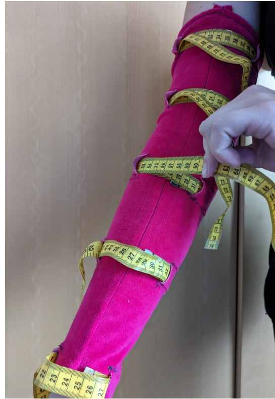
Figure 5.4: Prototype where the top 3 measuring tapes are tightened.
