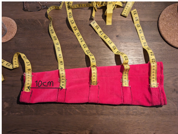
Figure 5.2: First testable prototype with measuring tape in a tunnel of stretch fabric.
