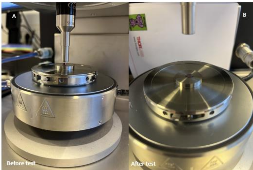
FIGURE 18: 20 G/L ALGINATE + 10% W/V IRON BEAD IN 100% CM BEFORE AND AFTER RHEOMETER TEST
