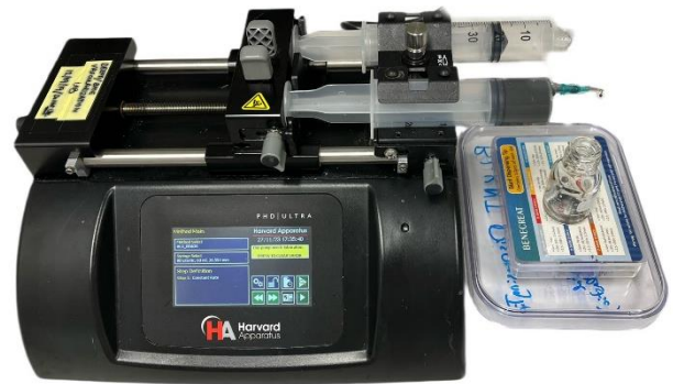
FIGURE 4: SET-UP OF HARVARD APPARATUS PHD ULTRA SYRINGE PUMP WITH 23G NOZZLE TO PRODUCE BEADS.
