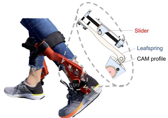
Fig. 1: A photo of the inGAIT-AFO being worn. Enlarged is an illustrated version of the leafspring-CAM mechanism including the adjustable slider. Figure partially taken from Bayón *et al.* [20].
