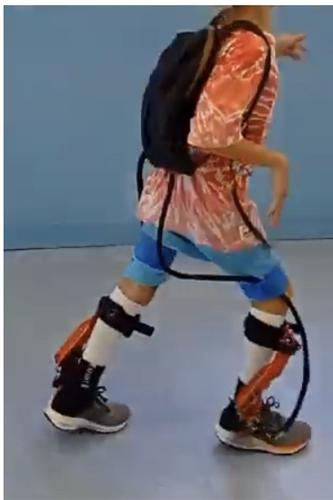
Fig. 9: A photo of a participant wearing the version 1 system during pilot testing
