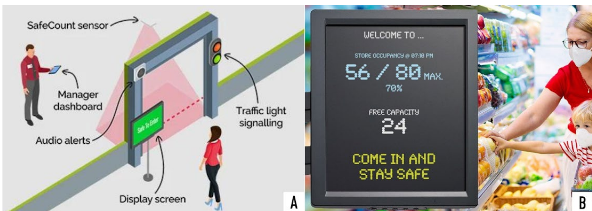
Figure 3. Examples of situated visualisations of occupancy data with digital signage: (A) diagram of Irisys SafeCount live occupancy monitoring system with visual warnings and alerts when limits are approached or exceeded [26], (B) Dilax live occupancy monitoring display showing the maximum store capacity, free capacity, and an alert indicating that it is safe to enter the building [27].
