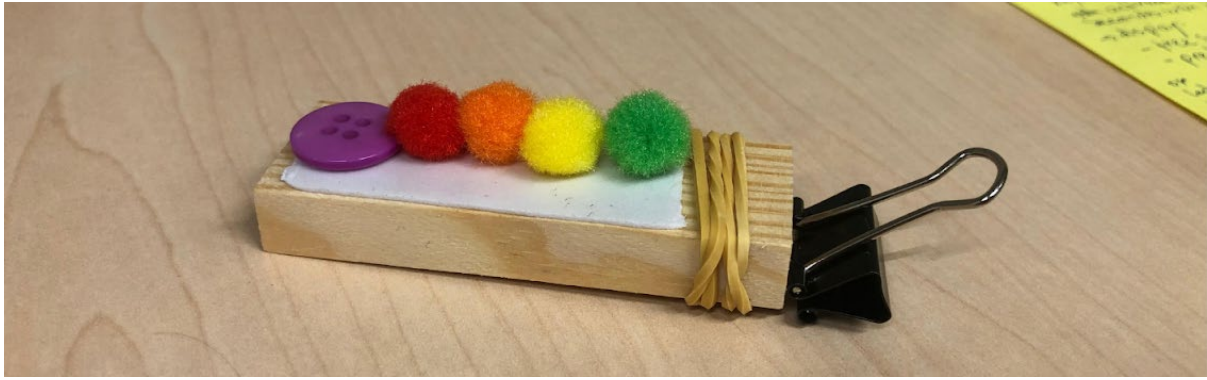
Figure 27. Light keychain: a physicalization equipped with vertically aligned LEDs that light up in colours from red to green based on the library’s occupancy, activated by a button (purple bead) press.
