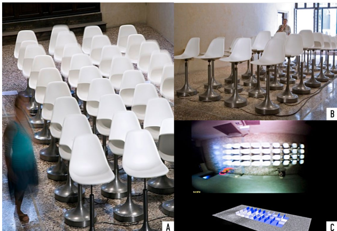
Figure 9. Wavefunction installation [38]: (a) shows the installation from above showing the four rows of chairs, (b) demonstrates the installation from the side with some elevated chairs, (c) displays the camera view and application that is used to sense the passersby and actuate the elevating chairs.
