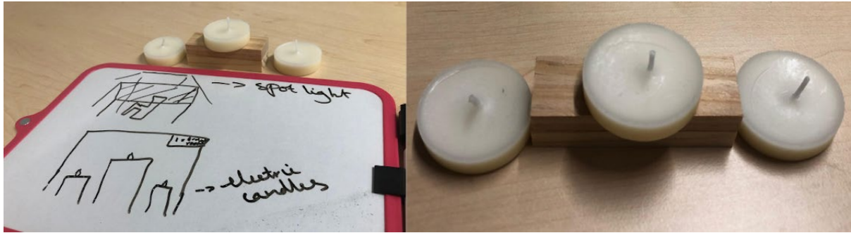
Figure 30. Candle display: left image) whiteboard drawing with an explanation of the physicalization idea, indicating a desk-size display featuring electric candles representing project rooms, where the candle is illuminated to indicate the room occupancy, right image) close-up view of the low-fidelity prototype created with tea lights.
