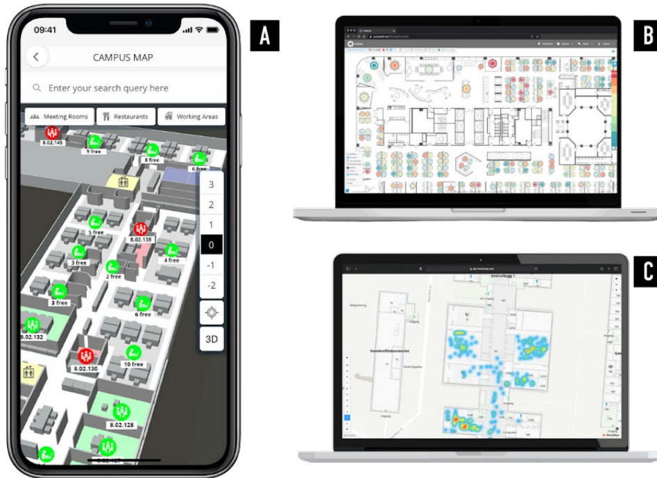
Figure 6. Examples of apps that indicate building occupancy on digital maps: (A) displays the infsoft Workplace Experience app showing current room utilisation in a 3D map [30], (B) demonstrates office occupancy heat map example of the CoWorkr software on a desktop [31], (C) shows other instance of an office occupancy heat map of the CoWorkr software [31].
