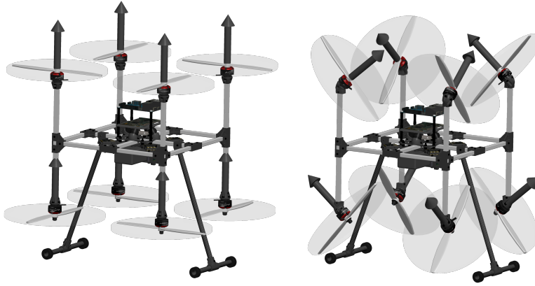
Figure 1.6: Model of the OmniMorph. Left: OmniMorph in the most energy-efficient rotor configuration by pointing all rotors directly upwards. Right: OmniMorph in the omnidirectional configuration, enabling it to hold its own weight in all possible poses. Credit: Aboudorra et al. (2024)
