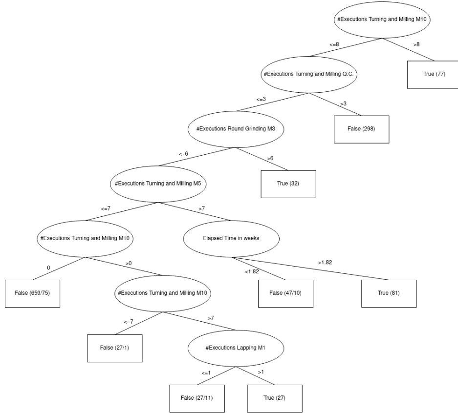
Fig. 1. This decision tree delineates the process feature classification for cable head production, identifying if rework is required ('True') or not ('False'). Each leaf node indicates the outcome ('True/False') along with the classification accuracy in the format (correctly classified/incorrectly classified instances).
