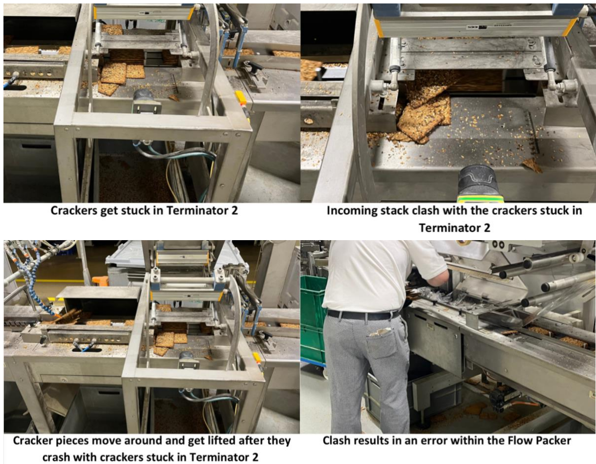
Figure 23 - Error within Flowpacker because of crackers being stuck in Terminator 2
