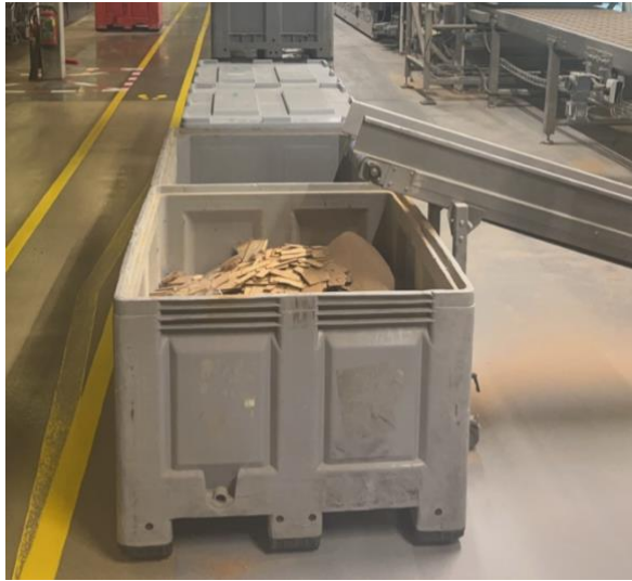
Figure 22 - Big box catching terminated crackers from the conveyor belt
