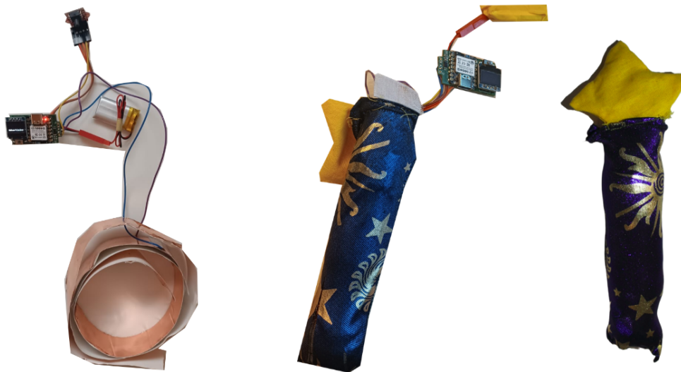
Figure E.8: A photograph of the hardware circuit (left), then with the balloon and the magic wand cover (middle), and with the microcontroller and battery in the star and thus finished (right).
