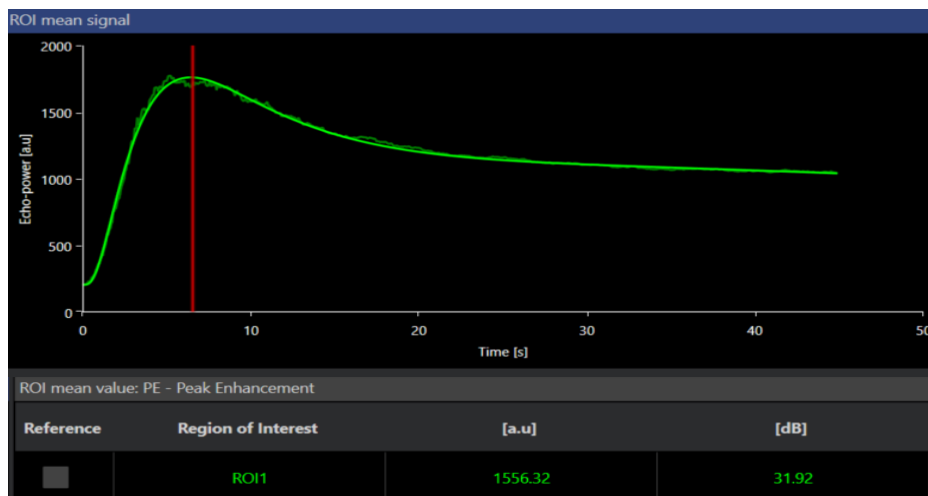
Figure 8. Example of a resulting TIC and PI output of Vuebox. A TIC is fitted by Vuebox over the intensity data from the point of microbubble arrival selected by the user. The resulting PI is given in an arbitrary unit, as well as in dB.
