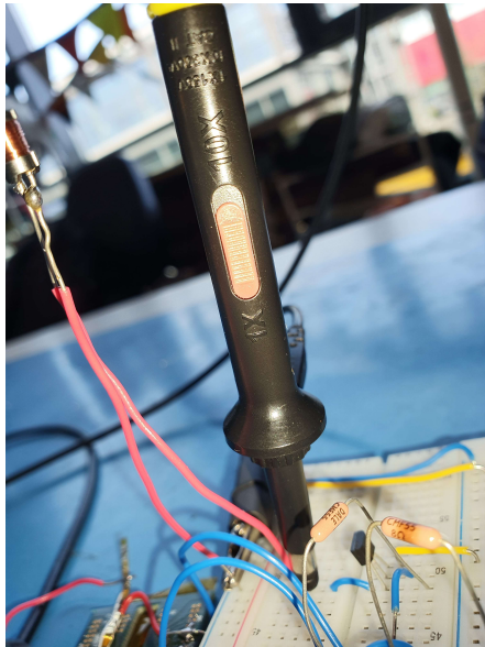
Figure 26: The probes which measured the voltage over the coils did not amplify the signal (amplification of 1x).
