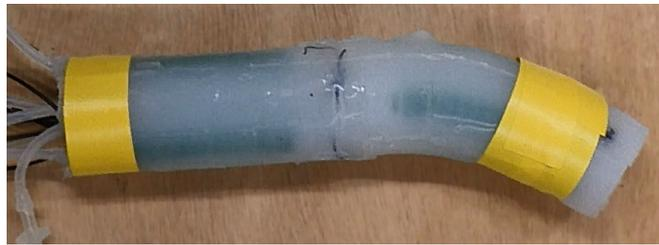
Figure 21: Full actuator, both modules inflated
