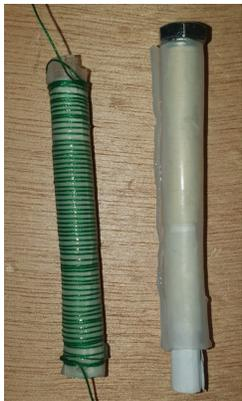
Figure A.1: Left: Fiber reinforced balloon,
