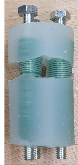
Figure B.3: First prototype, not enough silicon
