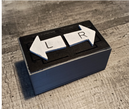
Fig. 10: A customized, wireless, 3D printed controller with left and right buttons.
