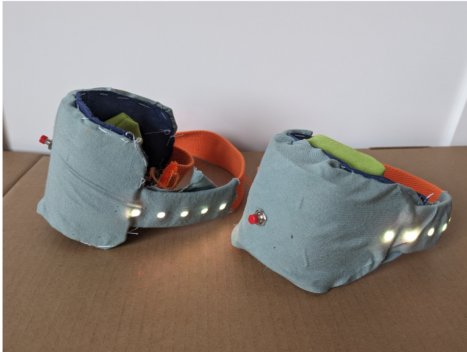
Figure 6.2: Final prototype with buttons, LED strip and wireless communication
