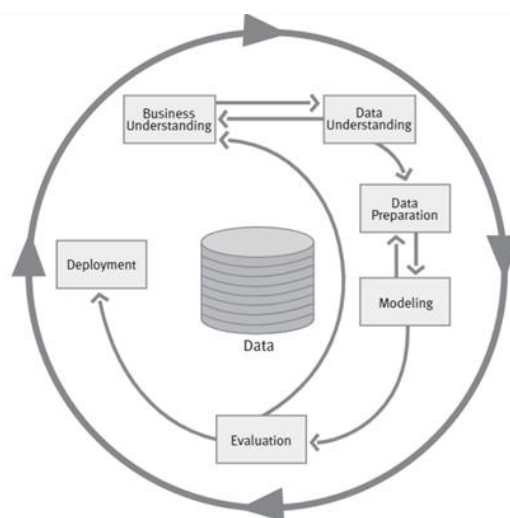
Figure 6: An overview of the CRISP-DM methodology adapted from Chapman (2000). The CRISP-DM methodology revolves around data. The figure shows the iterative process of creating data mining solutions. The methodology comprises business understanding, data understanding, data preparation, modeling, evaluation, and deployment.
