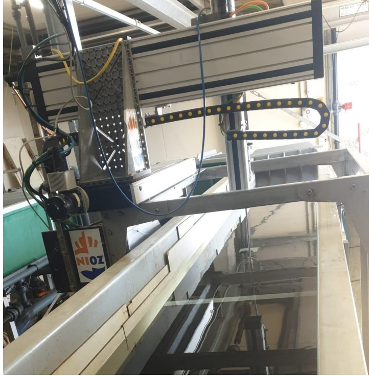
Figure 11: Carriage photographed from the upstream position looking downstream. The CNC arm is mounted on the left side of the carriage, the vertical axis of the arm positioned above the water has the ADV sensor attached to it. The legs on each corner have wheels mounted to be able to move the carriage between the various test sections.
