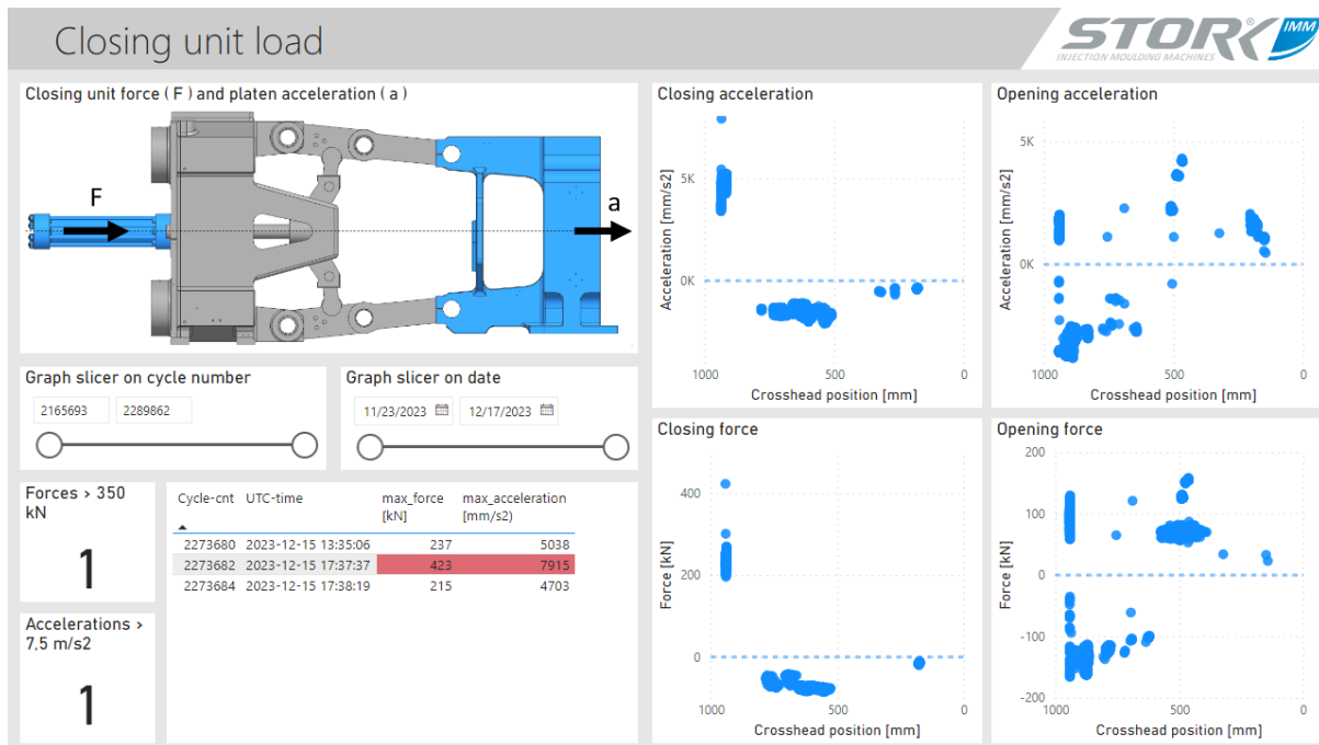
Figure 27, Dashboard frame load
