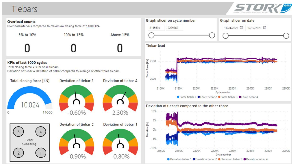
Figure 22, monitoring dashboard tie bars
