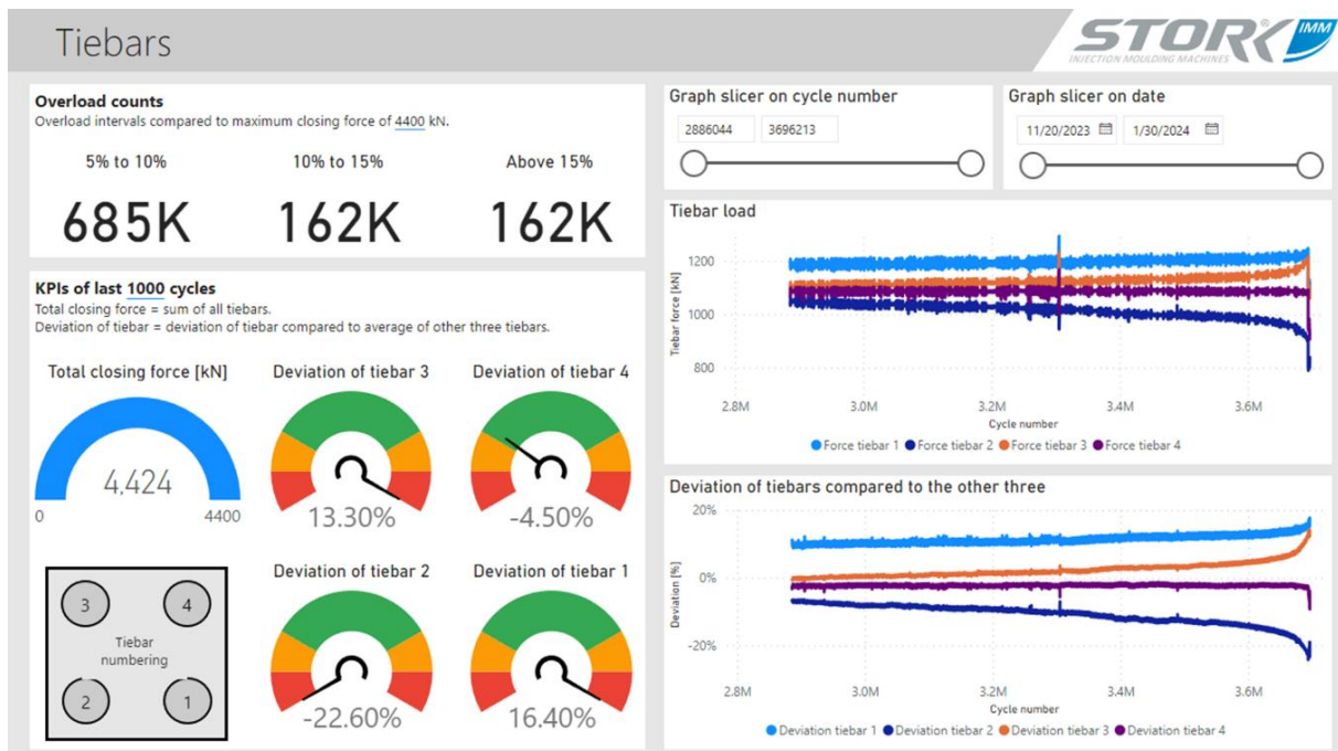
Figure 23, dashboard of a failing tie bar
