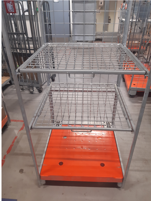
Figure 6: The roll container contains three compartments where the top two have the same dimensions and the bottom one is bigger.
