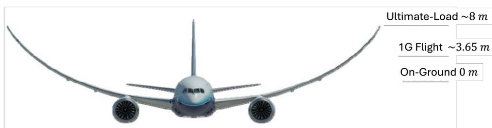
FIGURE 1.1 – Boeing 787 Dreamliner wing displacement under ultimate load conditions. Illustration from Dodt (2011) (edited).
