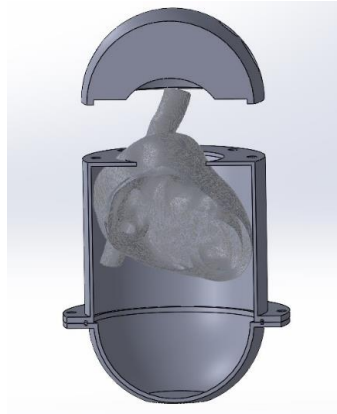
Figure 18 integration of heart model into the outer phantom using SolidWorks
