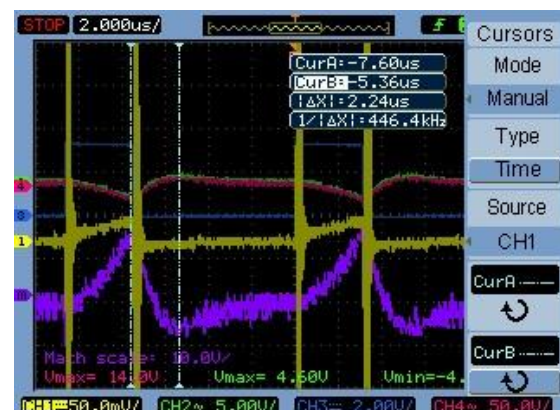
Figure 30b Green / pink showing the inverse voltage of the high side shunt, yellow showing the voltage over the low side shunt. Purple showing combined signal, representing the inductor current. Cursor shows t_{off}
