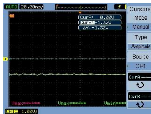
Figure 32 Yello line showing the 1.32 A DC current drawn from the battery. Minor noise at the left side of the signal is visable.
