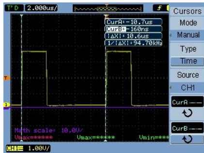
Figure 26 PWM signal showing a duty cycle of 30% with frequency of 94 KHz
