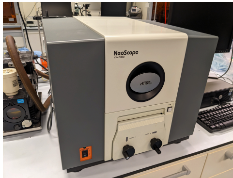
Figure 6.1: The NeoScope JCM-5000 used for taking the SEM pictures of the powders.
