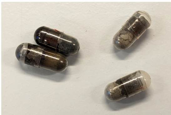
(a) All capsules, with neodymium on the left and permalloy on the right.
