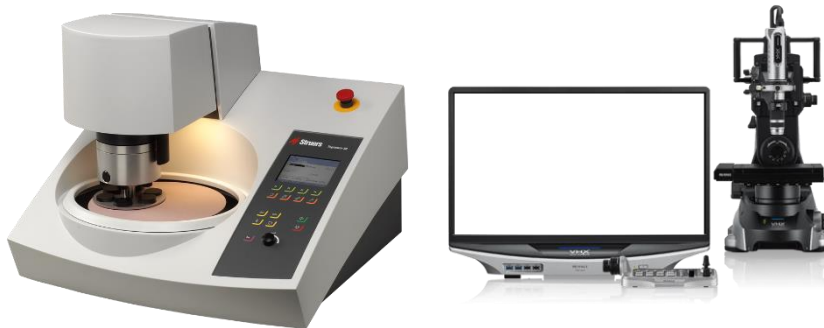
Figure 27. Equipment used for microscopic imaging Struers Tegramin-30 (left) [7] and Keyence VHX 7000 digital microscope (right) [12]
