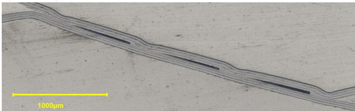
Figure 69. Cross section of an ultrasonic seal with four indents (sample 7 US)
