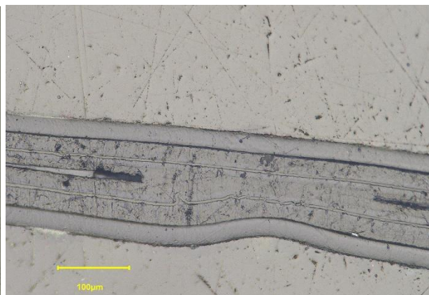
Figure 66. Disruption of the EVOH layer at one of the inner sealing sites (sample U6)
