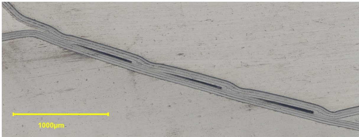
Figure 54. Microscopic image of ultrasonic seal cross-section (sample 7)
