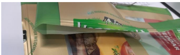
Figure 21. The side seal (conduction sealing) is open for a package (material 1 and 110°C)
