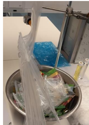
Figure 45. Transverse conduction seals stuck to each other
