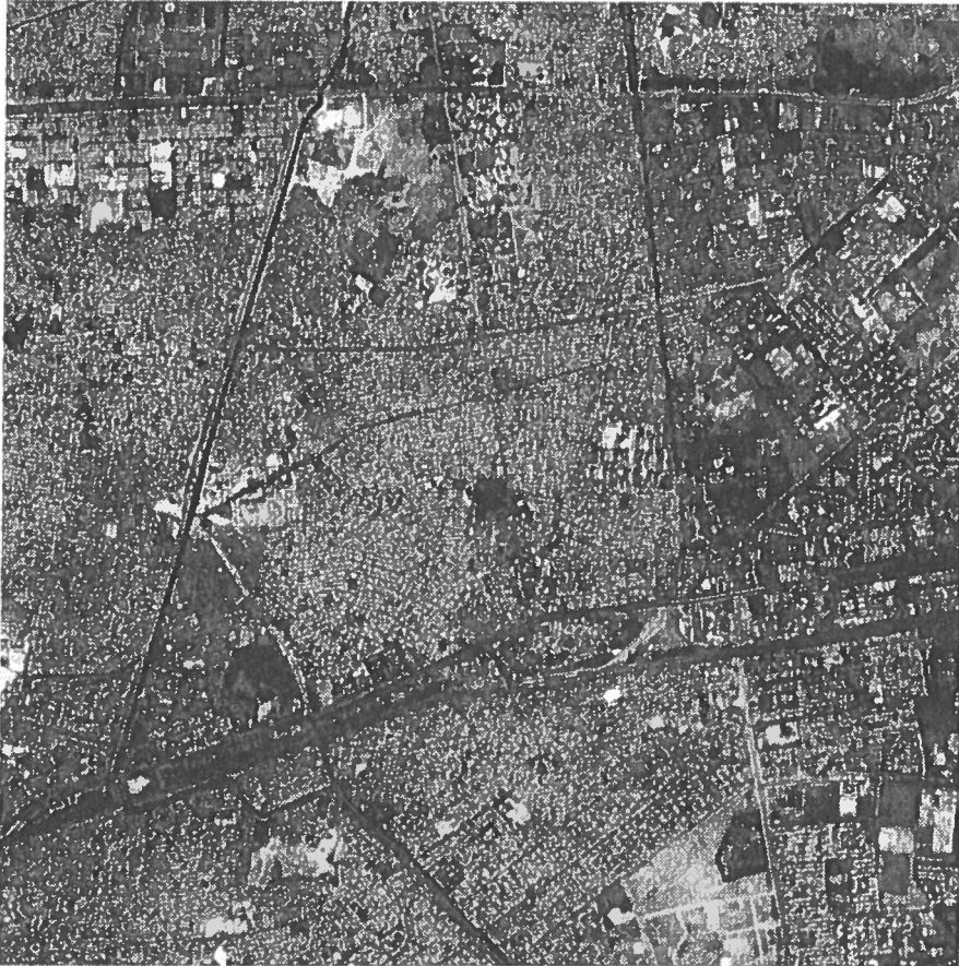
Figure 5.1 IRS-1C PAN image of the test site, east Delhi, used for segmentation. [1000x1000 pixels, Scale 1: 36,000]
